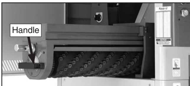
Figure 11. Spiral cutterhead access.
